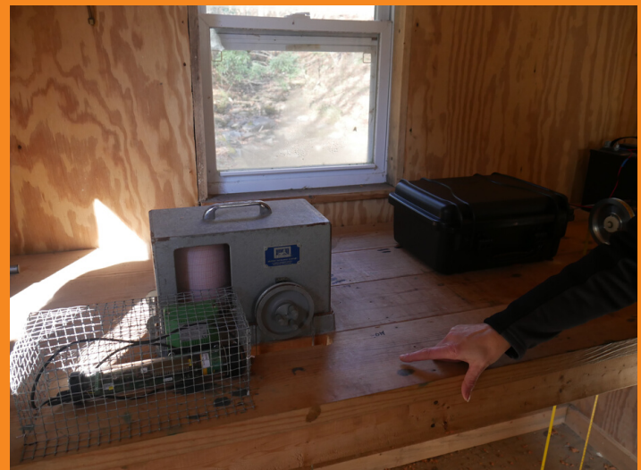
Tools used for measuring height of water in the pool; the recorded information is checked once a week.
